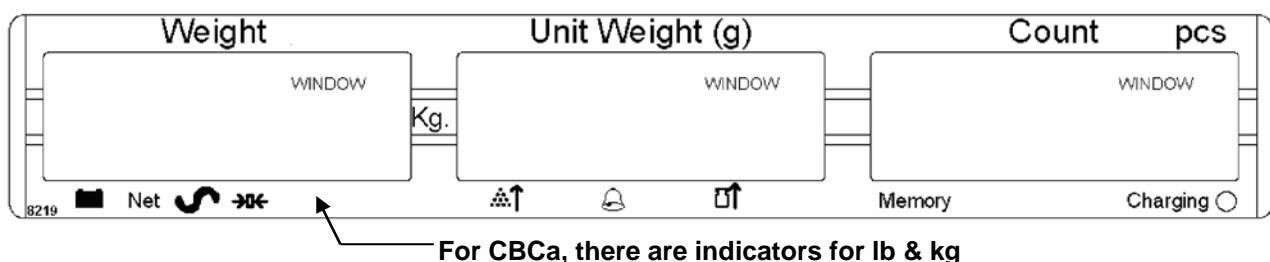
The scale will show the model No in the “Weight” display window (e.g: CBC 30- where 30 denotes the maximum capacity of the scale in Kg) and the current hardware and software revision numbers in the “Unit Weight” display window .Next a self-test is followed. At the end of the self-test, it will display “0” in all three displays, if the zero condition has been achieved.
